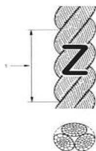
5A Z – lay or right – hand lay
