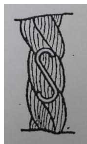
5B S – lay or left – hand lay
